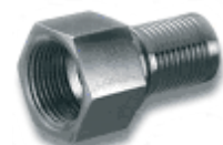
MALE OR FEMALE PIPE THREAD Male and female NPT or GAS pipe thread fittings are internally finished to sanitary quality and incorporate the internal chamfer feature.
